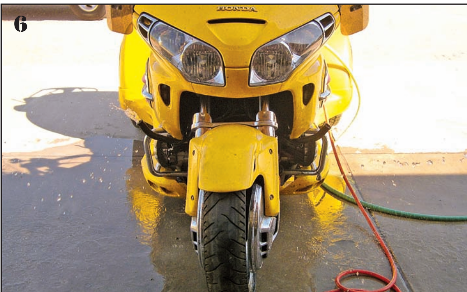
Pressure applied at cylinder head rear blasts through the front hoses.
